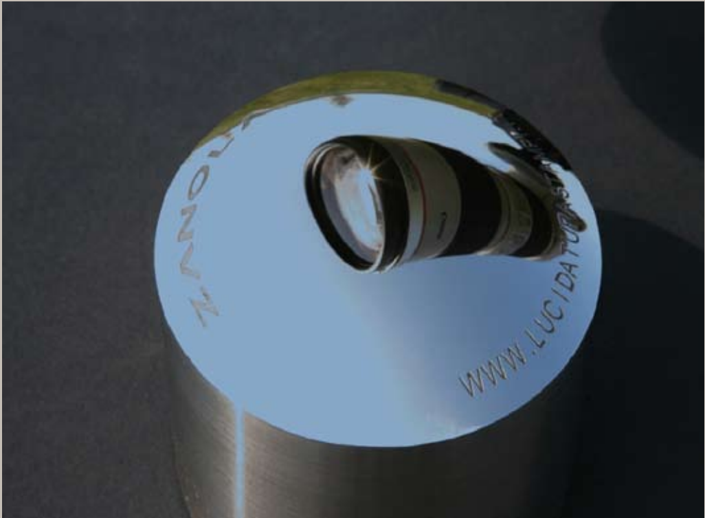
Figure 13. TOOLOX 33 polished to optical requirements.
