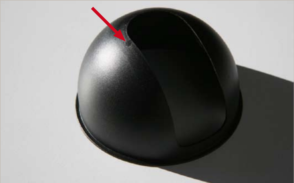
Figure 14. Imperfection on plastic surface generated by the ejector pin.
