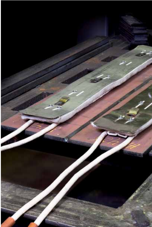
Figure 5: Example of electrical heating mats
