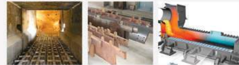
Clinker cooling guide plates Temperature around 500°C
