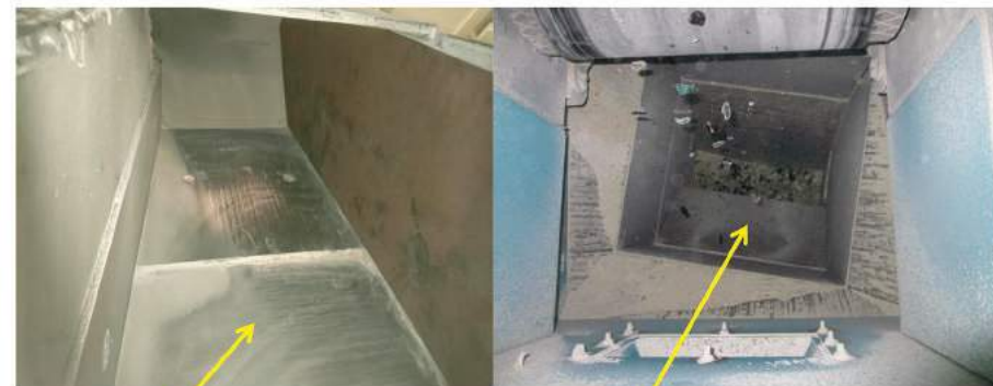
Hardox Extreme in chute Silo impact, vibrating/sorting table, Hardox 450 *Cleanliness very important!
