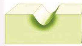
Micro cutting - High wear
