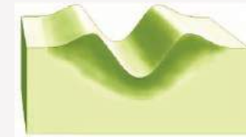
Micro ploughing - Low wear
